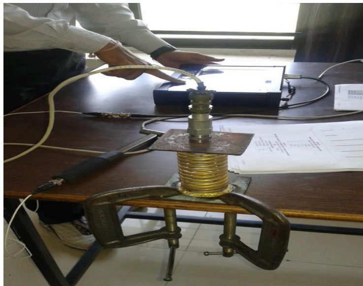
Fig. 8 Experimental setup for Brass spring
