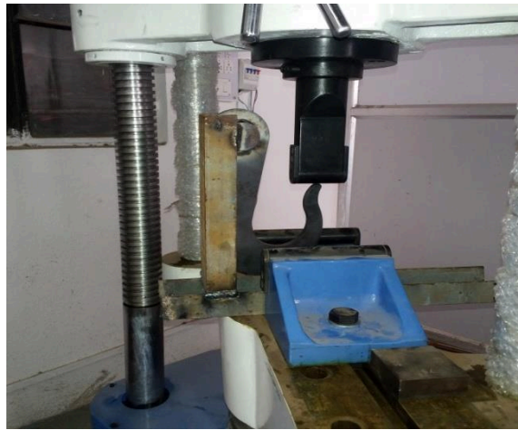
Fig. 10. Experimental testing of hook on UTM
