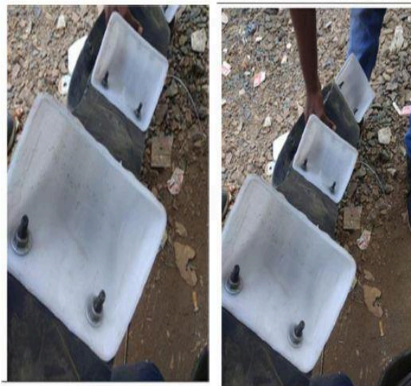
Fig.6 Belt Bucket Conveyor
