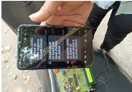
Fig. 8(ii)SMS through GSM
