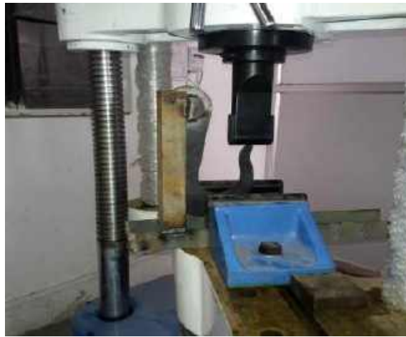
Fig. 10. Experimental testing of hook on UTM
