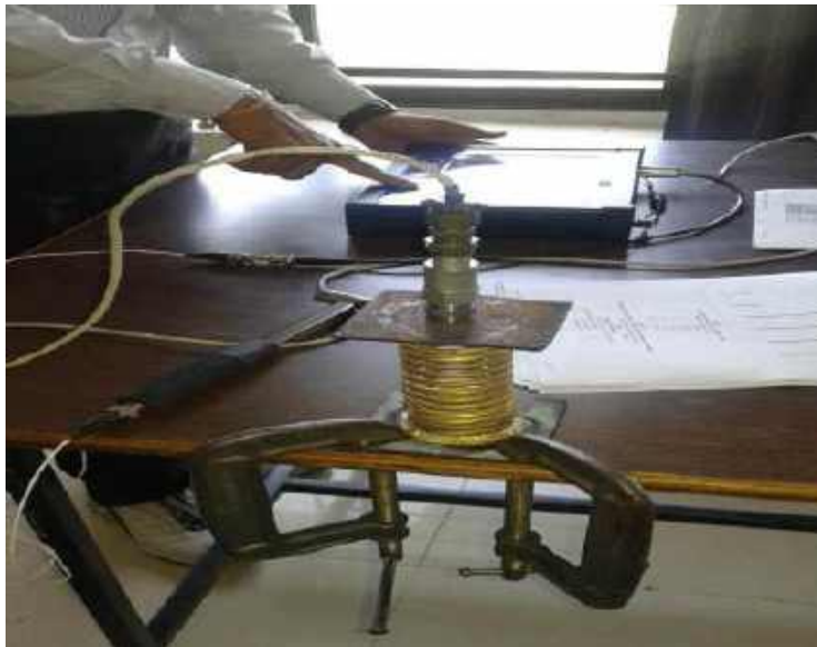
Fig. 8 Experimental setup for Brass spring
