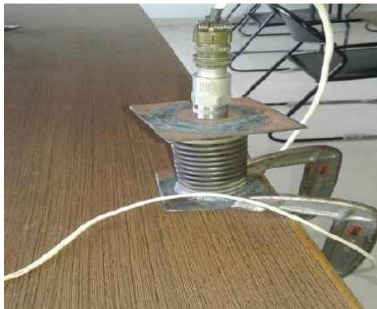
Fig. 7 Experimental setup for Steel spring
