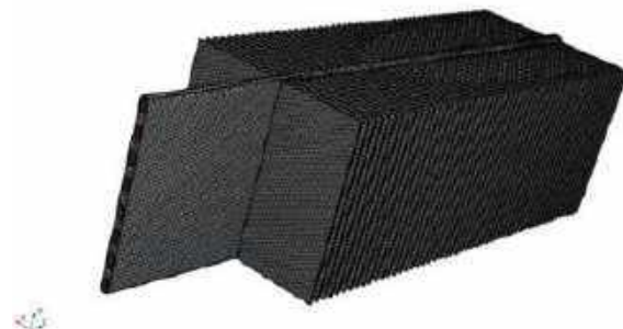
Fig. 5 Mesh Generation of Heat Exchanger
