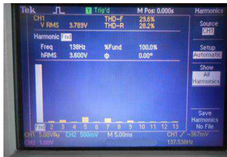
Fig. Harmonics generated by 5-level Inverter across resistive load
